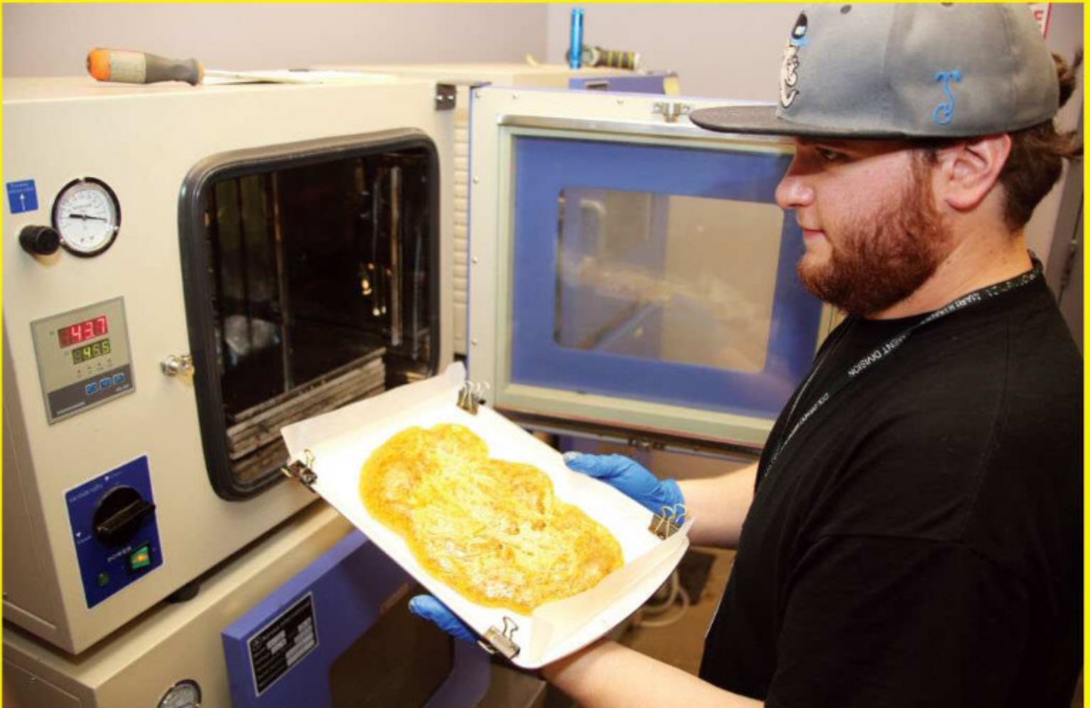
(Above and left) TC Labs uses laboratory vacuum ovens for the next step in the process. The oven introduces heat and pressure to remove the solvent left in the solution. The butane and hash solution will "boil" as the remaining solvent continues to release its bonds.
